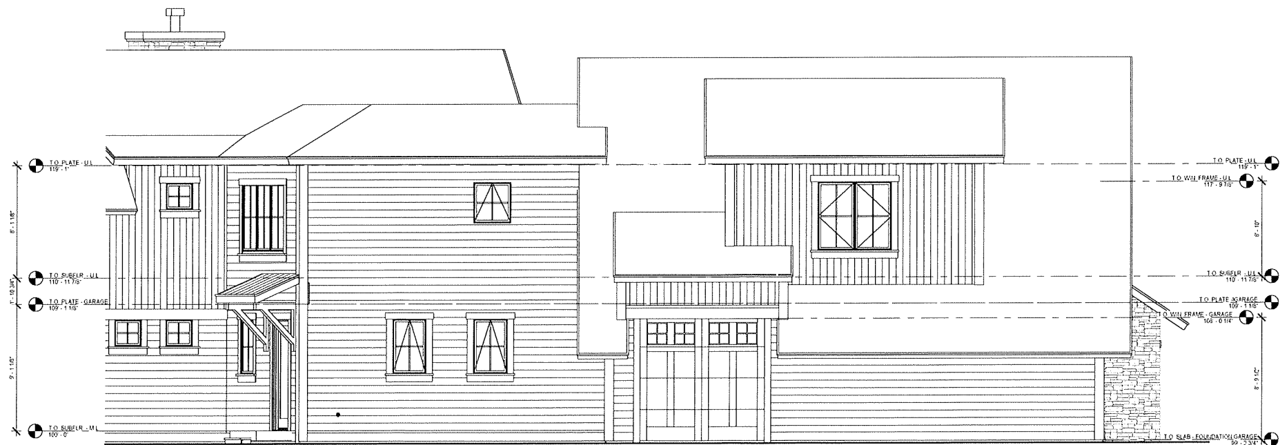
3 GARAGE WEST ELEVATION A2.3 1/4" = 1'-0"
